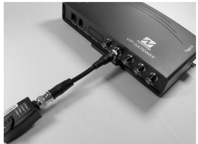
Fig. 13: Video balun connected to gateway using the BNC patch cable.
